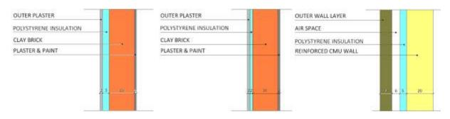
**Figure 7.** Types of walls to be compared. Left traditional wall with 5cm. insulation, middle traditional wall with 2 cm. insulation, right NP 12's wall system.
