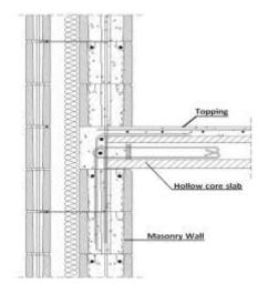
Figure 3: Typical hollow core slab, masonry wall connection.
